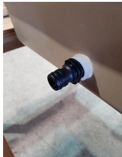
Male fitting shown correctly in plastic tub.
