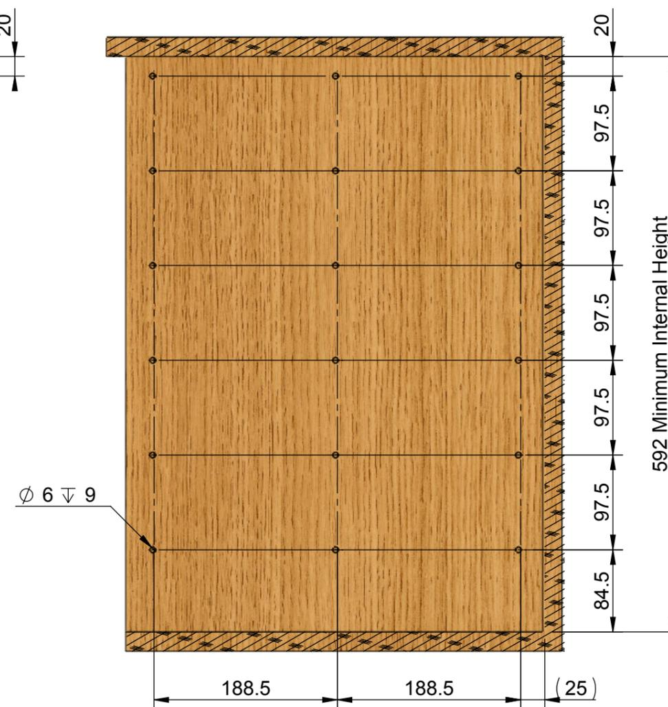
Section view showing machining detail for location hole centres.
