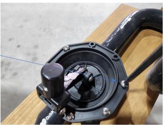
STEP 6: Remove the flange housing from the pump.
