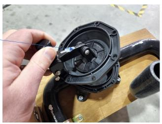
STEP 5: Remove the centre screw holding the flange on.
