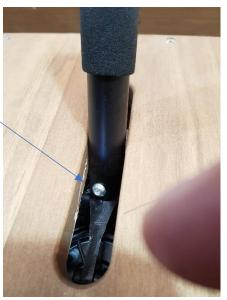
STEP 3: Remove the 3 wood screws at the bottom of rear plate.
